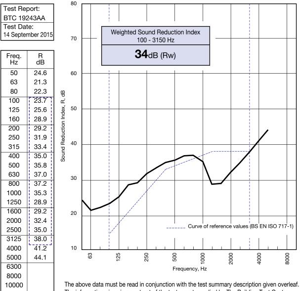
The information given is an extract of the test report supplied by The Building Test Centre, East Leake, Loughborough. BTC is a UKAS approved test laboratory.
