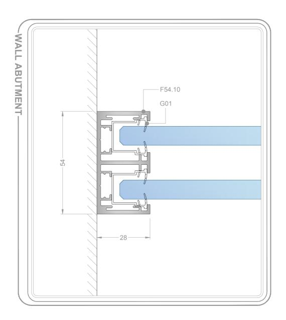
Drawing Title Fineline D/Glazed Head Channel Abutment Scale @ A4 Drawn by Checked 1:1 S.BM - Date Unless stated 20/03/17
