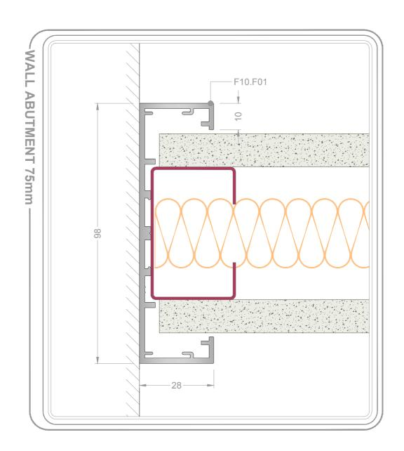
Drawing Title Fusion 10 - Solid 75mm Head Channel Abutment Scale @ A4 Drawn by Checked S.BM 20/02/17
