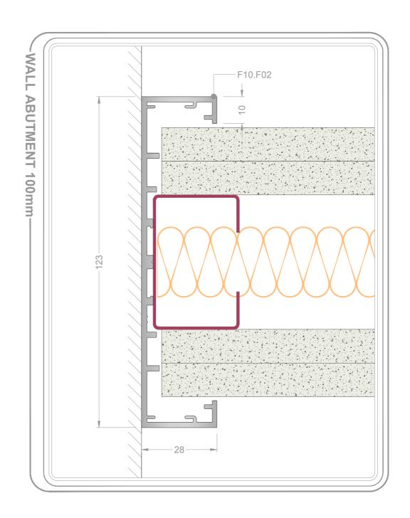
Drawing Title Fusion 10 - Solid 100mm Head Channel Abutment Scale @ A4 Drawn by Checked 1:1 S.BM - Date 20/02/17
