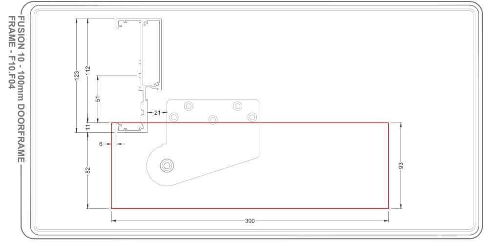
Floor box cutout Contempo - Frame F10.F04 Scale @ A4 Drawn by Checked 1:2 unless stated S.BM -Date 24/07/20 Rev.
