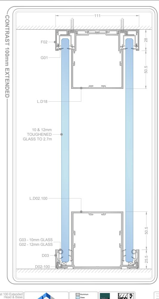
Drawing Title Contrast 100 Extended Head & Base Scale @ A4 Drawn by Checked NTS S.BM - Date 20/02/17 Drawing no. Rev.
